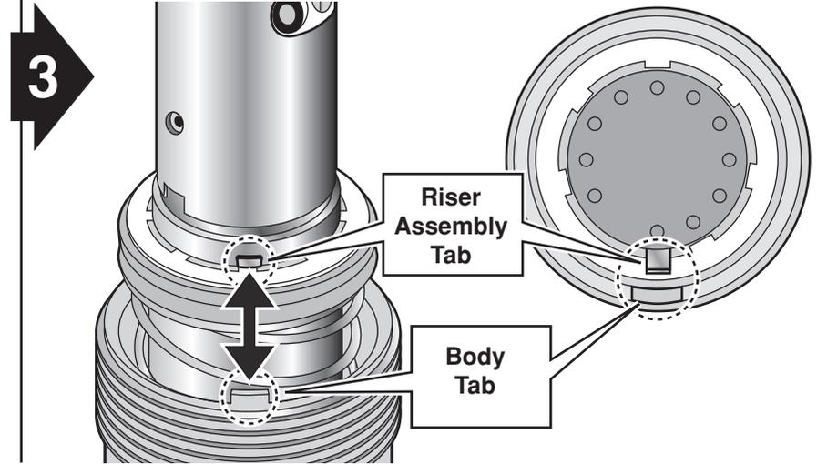
**3** Insert riser assembly into body. Align riser assembly tab with body tab as shown.
