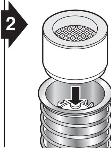
**2** Press stator assembly into bottom of riser assembly.
