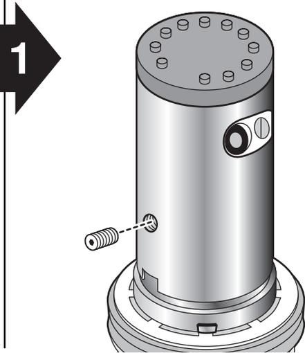
**1** Thread nozzle turret onto riser assembly and secure with 1/16" hex set screw.
