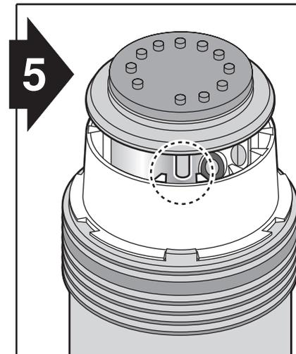
**5** Install nozzle seal with boss inserted between guide ribs.
