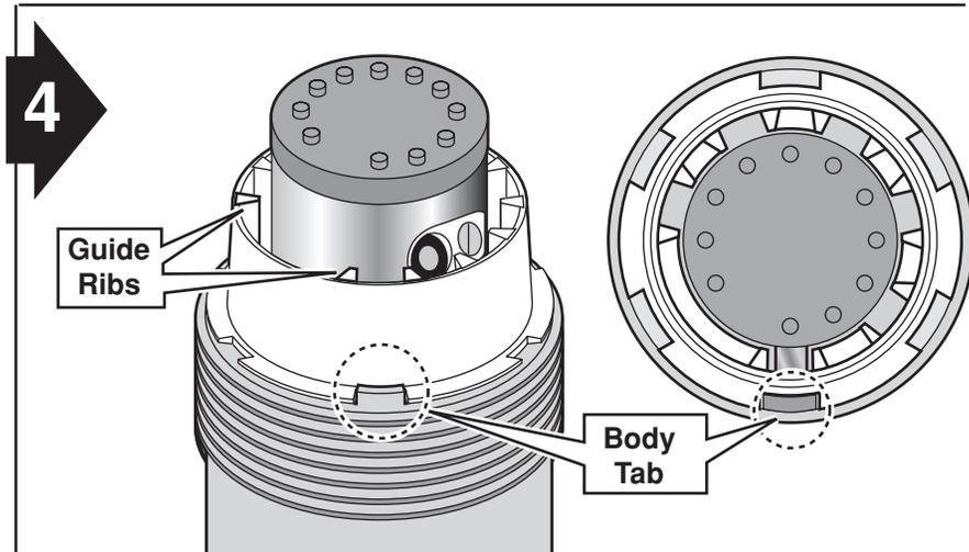
**4** Insert nozzle retainer into body. Note spacing of guide ribs and align with riser assembly tab and body tab as shown.
