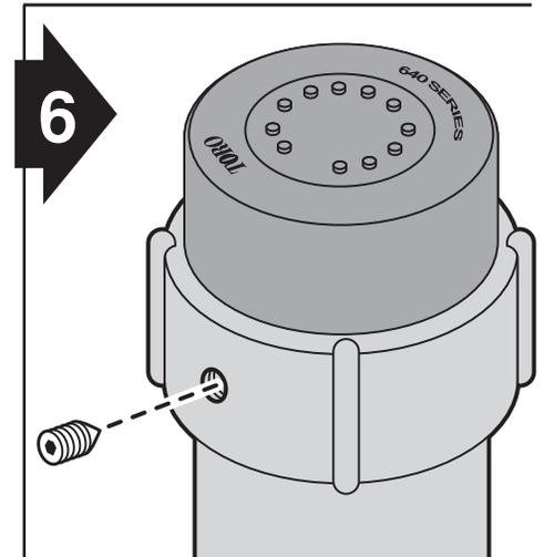
**6** Install cap and secure with 1/8" hex set screw.
