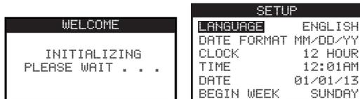
Upon power up, the initialization screen will display briefly. On initial power up, the EVOLUTION™ will display the SETUP screen. This SETUP screen is only accessed during initial power up or after a factory reset is performed.
